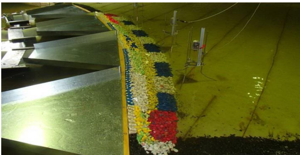
Figure 5 Physical Modelling of the Preferred Primary Upgrade Option
